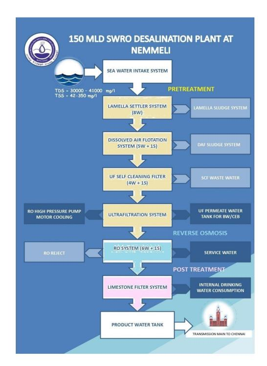
Lamella clarifier is designed for clarification of water to reduce the TSS content to permissible limit. The seawater flows up in the direction opposite to gravity through the lamella plates after the coagulation and flocculation stages. The heavier floc settles on the inclined plates and gets collected in the bottom hopper. Flotation is a process of liquid-solid separation by upward displacement of particles insoluble in water, under the action of the field of gravity. Membrane filtration
