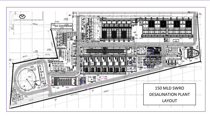
This work involves Seawater intake system, Pre-treatment units, RO plant with energy recovery system, post treatment units, reject disposal system, Product water tank and connected Pump House for transferring the Product Water. Sea Water Quality considered for the design of the facility
